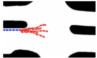
Figure 4.2: Task input and outputs. The binary drivable area is represented as the black-and-white bird eye view, the past trajectory in blue and the N future trajectories in red.
