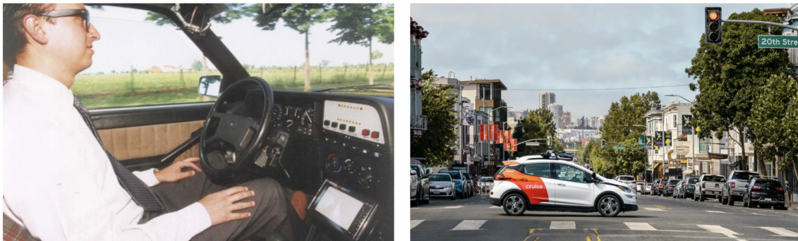
Figure 1.1: Autonomous driving systems historical landmarks. (left) the interior of a Mercedes W140 S-Class, re-engineered in the context of the Prometheus project, which drove 1,678 kilometers from Munich to Copenhagen with minor human intervention. (right) A Cruise autonomous robotaxi in the streets of San Francisco, June 2022.
