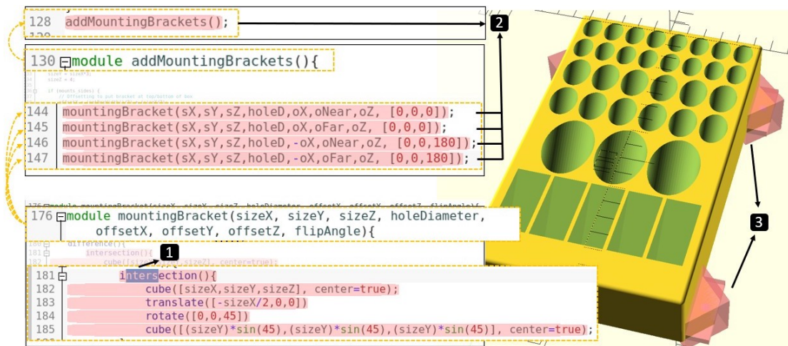
Figure 22: Forward navigation features. F4 : After selecting a portion of an instantiating statement, (1) all the instance creations of the selected code are highlighted in pink, and (2) all the resulting elements are highlighted in pink in the 3D view (3).
