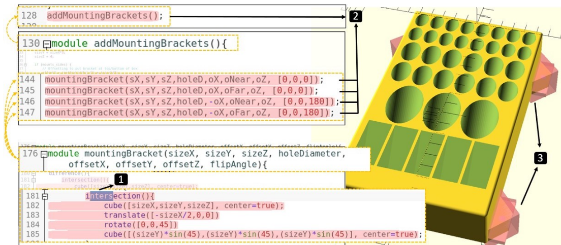
Figure 22: Forward navigation features. F4 : After selecting a portion of an instantiating statement, (1) all the instance creations of the selected code are highlighted in pink, and (2) all the resulting elements are highlighted in pink in the 3D view (3).
