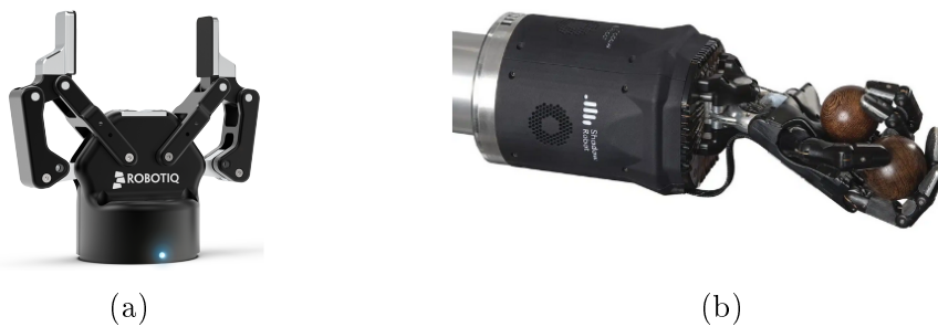
Figure 2.6: Robotic manipulators: (a)RobotiQ gripper (b) Shadow hand
