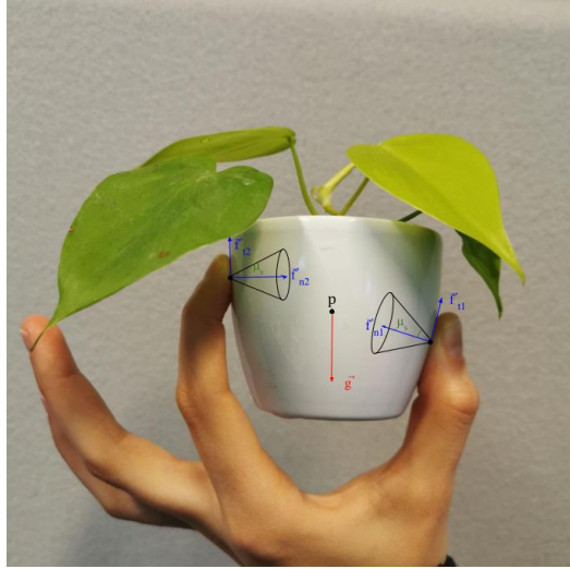
Figure 3.1: Forces acting on a grasped object. The two fingers apply a normal force on the object f_{n1} and f_{n2} at both contact points that, in the absence of disturbance, compensate for the gravity acting on the object. The friction cone must contain the resultant force vector to prevent slip. Note that the two cones have different dimensions, as each finger independently applies the forces.
