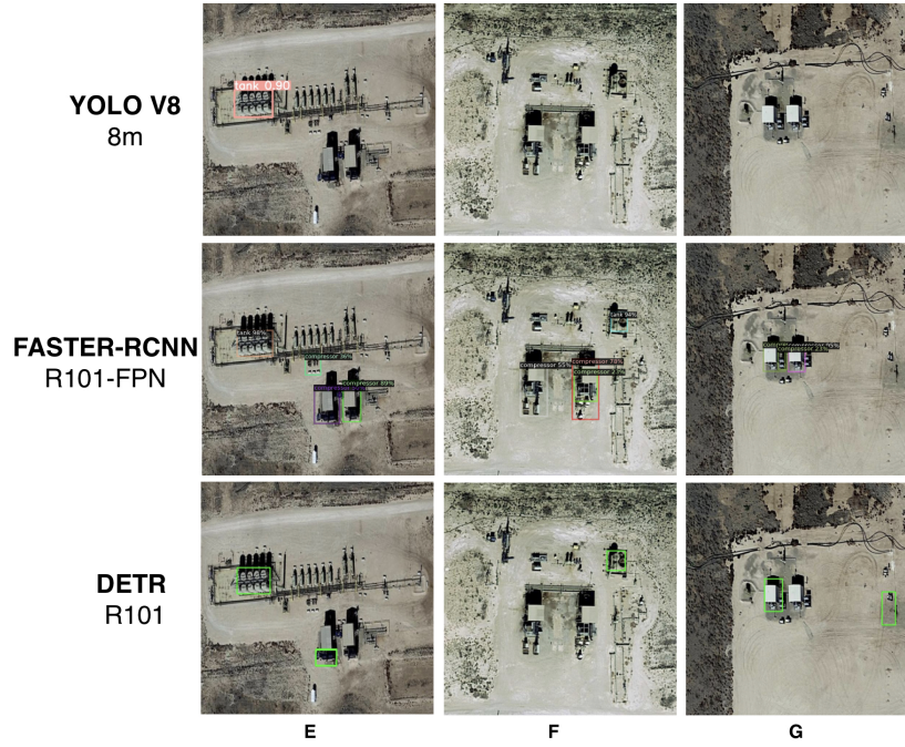
Figure 3.11: Comparison of pre-trained YOLO v8, FASTER-RCNN and DETR on a special (less representative) compressor architecture in the Permian Basin (images sources @Google Earth).
