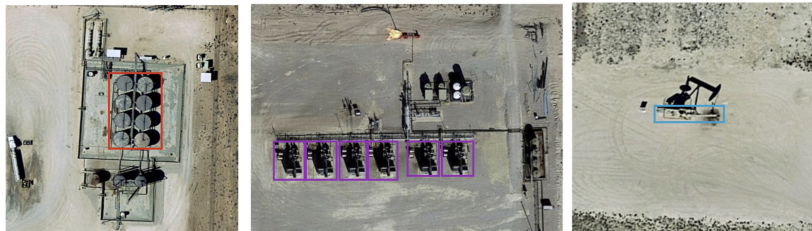
Figure 3.4: Example of images and annotated objects from OG database : tank (red), compressor (purple) and well (blue) source : @Google Earth.
