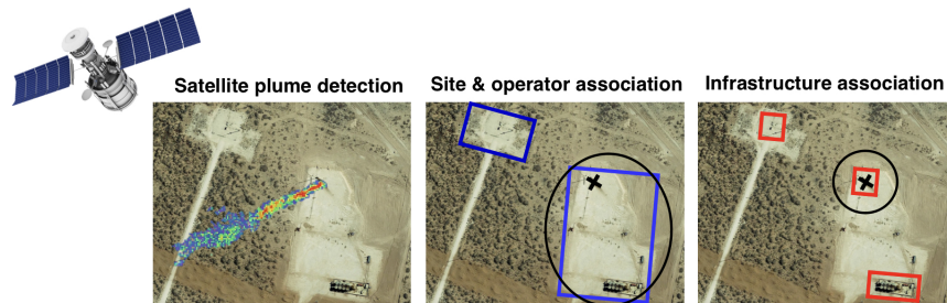
Figure 4.1: Detected Methane plume association to O&G site, operator and infrastructure by spatial location. Source : @Google earth.
