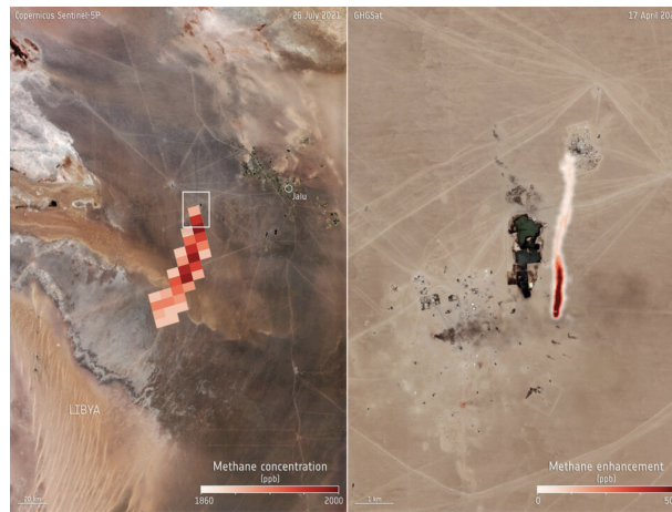
Figure 2.7: Methane plume enhancement over Libya by Satellites TROPOMI Sentinel 5P and GHGSat Image source: European Spatial Agency.
