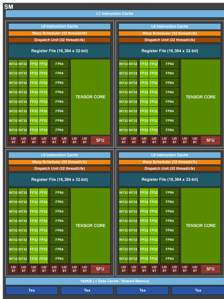
(b) Streaming Multiprocessor (SM) architecture
