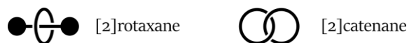
Figure 1.4. Two families of mechanically interlocked molecules: rotaxanes, where a macrocycle surrounds an axle, and catenanes, where macrocycles interpenetrate each other.
