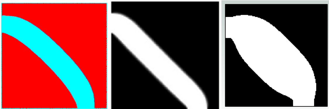
(a) Optimized domain [140] for 90° pipe bend using the shape optimization (b) Optimized domain [130] for 90° pipe bend—rotated 90° counter-clockwise (c) Optimized domain (inhouse code result) for 90° pipe bend—rotated 90° counter-clockwise
