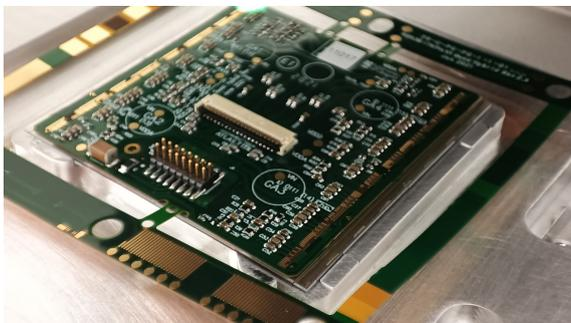
Figure 3.2.3: The 3D-printed jig for the Pixel module fixation under the microscope.
