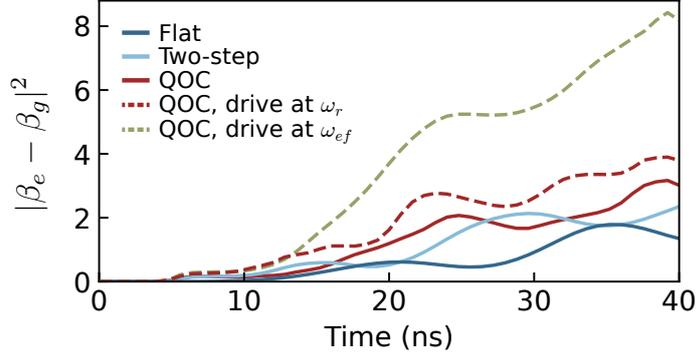
Figure 4.6: Phase space distance in the Purcell filter mode between  $|g\rangle$  and  $|e\rangle$  transmon states against time, for a 40 ns readout and for various reference and optimized pulses. The SNR is the integral of this quantity, up to some multiplicative factor.
