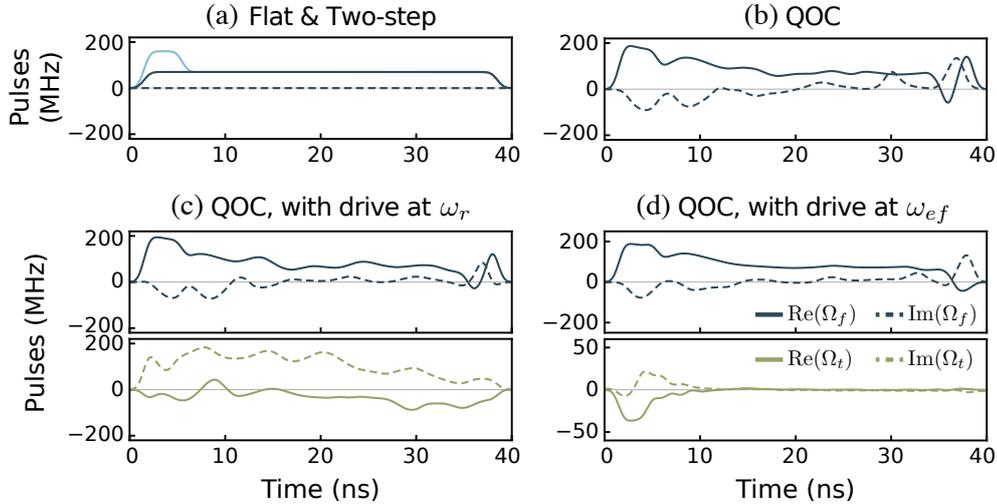
Figure 4.5: Example of various reference and optimized pulses for a 40 ns readout. Solid and dashed lines show the real and imaginary parts of (4.24) respectively. (a) Flat (dark blue) and two-step (light blue) pulses. (b) Optimized readout pulse. (c) Optimized readout pulses with a transmon drive at  $\omega_{d,t} \approx \omega_r$ . (d) Optimized readout pulses with a transmon drive at  $\omega_{d,t} \approx \omega_{ef}$ .
