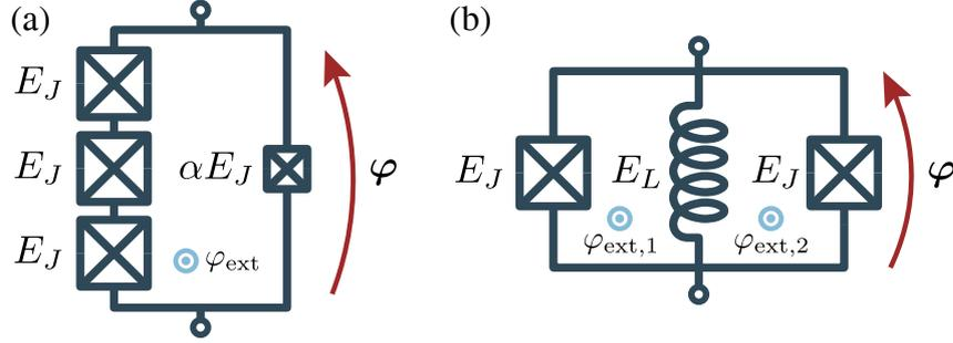
Figure 1.7: (a) Lumped-element circuit of a SNAIL with  $n = 3$ , used to engineer Kerr cat qubits. Figure adapted from [Frattini *et al.* 2017]. (b) Lumped-element circuit of an ATS, used to engineer dissipative cat qubits. Figure adapted from [Lescanne *et al.* 2020b].
