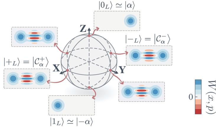
Figure 1.4: Encoding a cat qubit in a quantum harmonic oscillator. Computational states on the  $Z$  axis of the Bloch sphere are approximately coherent states delocalized on either side of phase space, hence providing an exponentially small probability of bit-flip errors.
