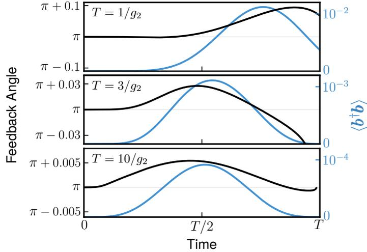
Figure 3.6: (Black) Angle of the  $Z$  rotation feedback to perform after a buffer mode photodetection at any given time, for a  $Z(\pi)$  gate of duration  $T$ . (Blue) Buffer mode population for the no-jump trajectory, proportional to the photodetection probability  $\langle dN_\eta \rangle$ . In these numerical simulations,  $\kappa_b = 8g_2$  and  $|\alpha|^2 = 8$ .
