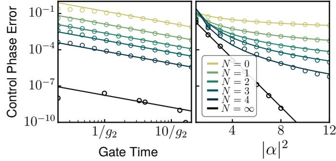
Figure 3.10: Gate-induced control phase errors for a CNOT gate with a locally flat drive Hamiltonian as in (3.26). Left: fixed cat size,  $|\alpha|^2 = 8$ . Right: fixed gate time  $T = 10/g_2$ . Dissipative stabilization is acting on the control qubit only, with  $\kappa_b = 8g_2$ . Lines show numerical fits of the form  $p_{Z_C} \propto T^{-1}|\alpha|^{-2N}$  (color) and  $p_{Z_C} \propto T^{-1} \exp(-2|\alpha|^2)$  (black). Markers show numerical data.
