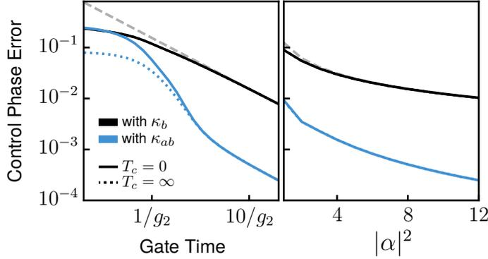
Figure 3.8: Gate errors of a CNOT gate with the autonomous feedback design of (3.14) at  $\kappa_{ab}/|\alpha|^2 = 8g_2$  (blue) and with the regular Zeno design at  $\kappa_b = 8g_2$  (black). Left: fixed cat size,  $|\alpha|^2 = 8$ . Right: fixed gate time,  $T = 10/g_2$ . Gate errors are evaluated at  $t = T$  or after full reconvergence to the steady state ( $T_c = \infty$ ). Dashed gray lines show analytical CNOT gate errors [Chamberland *et al.* 2022].
