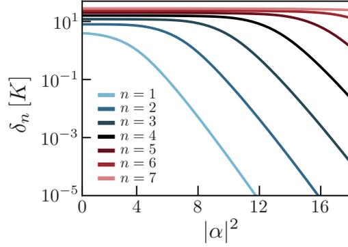
Figure 2.3: Energy level spacing between even and odd parity eigenstates of the Kerr Hamiltonian  $\delta_n = |e_n^- - e_n^+|$ . Similar plot as in Figure 2.2(a) but with a logarithmic scale on the vertical axis.
