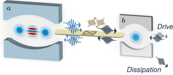
Figure 1.8: Schematic of a cat qubit mode  $a$  stabilized by a two-to-one photon exchange with buffer mode  $b$ , mediated by a nonlinear circuit element (middle) and a pump at the appropriate differential frequency. The buffer mode is driven and dissipates photons to the environment.
