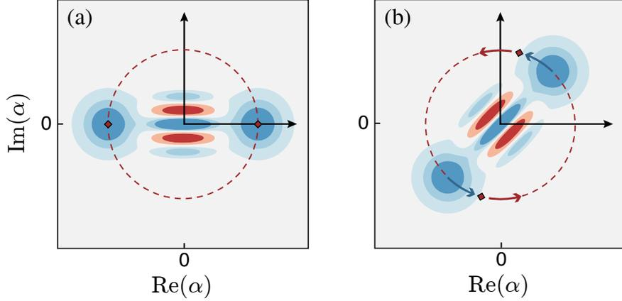
Figure 1.11: Codespace deformation. (a) Idling cat qubit, with fixed points of the confinement in  $\pm\alpha$  (red diamonds). (b) Codespace deformation during an  $X$  gate. The confinement fixed points are rotated along the red circle. The cat qubit is "pulled" towards these fixed points for sufficiently slow rotations. Figure adapted from [Guillaud & Mirrahimi 2019].
