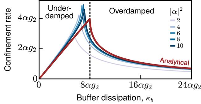
Figure 1.9: Confinement rate  $\kappa_{\text{conf}}$  of a dissipative cat qubit as a function of the buffer mode dissipation rate  $\kappa_b$ . The maximal confinement rate  $\kappa_{\text{conf}}^* = 4\alpha g_2$  is obtained at the critical regime for  $\kappa_b = 8\alpha g_2$ . The red line is obtained from semiclassical analysis. Blue lines are obtained from exact diagonalization of the Liouvillian.
