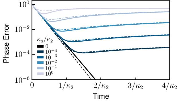
Figure 3.12: Gate-induced phase errors of a discrete  $Z(\pi)$  gate as in (3.35) with additional single-photon losses of the form  $\kappa_q \mathcal{D}[\sigma_-]$  on the ancillary qubit. Dashed lines show  $p_Z = \kappa_q t + \exp(-|\alpha|^2 \kappa_Z t)$ . The cat size is fixed at  $|\alpha|^2 = 8$  and  $\kappa_Z/\kappa_2 = 1$ .
