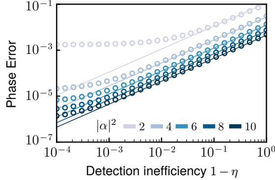
Figure 3.5: Scaling of phase errors of a  $Z(\pi)$  gate against detection inefficiency  $1 - \eta$ , for increasing values of  $|\alpha|^2$ . Gate errors are evaluated at  $t = T = 4/g_2$  without reconvergence ( $T_c = 0$ ). Markers show numerical integration of the SME with classical feedback. Solid lines show (3.13), with a linear scaling with  $1 - \eta$ . In this numerical simulation,  $\kappa_b = 8g_2$ .
