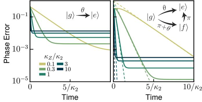
Figure 3.13: Gate-induced phase errors of a discrete  $Z(\pi/3)$ , with the designs of (3.35) using an ancillary two-level system (left) and of (3.40) using an ancillary three-level system (right). Dashed lines show  $p_Z = \exp(-|\alpha|^2 \kappa_Z t)$ . Insets show the gate transitions between ancillary states for either design.
