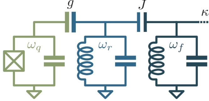
Figure 4.3: Lumped-element circuit of a transmon-resonator-filter model. The transmon (green) and readout resonator (blue) are capacitively coupled with coupling  $g$ . The resonator is itself capacitively coupled to a Purcell filter (dark blue) with coupling  $J \ll g$ . This filter is damped and driven through a transmission line.
