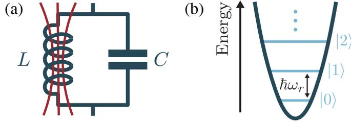
Figure 1.1: (a) Lumped-element model of a LC resonator with inductance  $L$  and capacitance  $C$ . (b) Harmonic oscillator potential with resonant frequency  $\omega_r$ . Figure adapted from [Blais *et al.* 2021].
