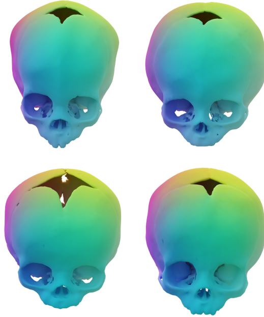
Figure 4.6: Visualization of computed correspondences between two random pairs of shapes in the collection. Top : correspondence between two nearly isometric scans. bottom : correspondences between highly non-isometric scans. Vertices on the left are given RGB colors depending on their XYZ coordinates, and corresponding vertices between left and right are given the same color.
