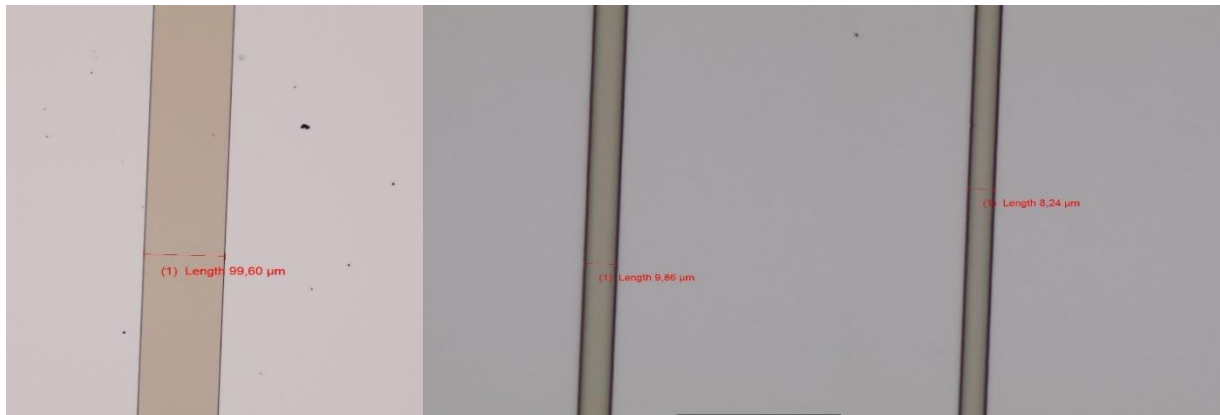
Figure 3.12. Photo from optical microscope of mesas with widths of 100 μm, 10 μm, 8 μm
