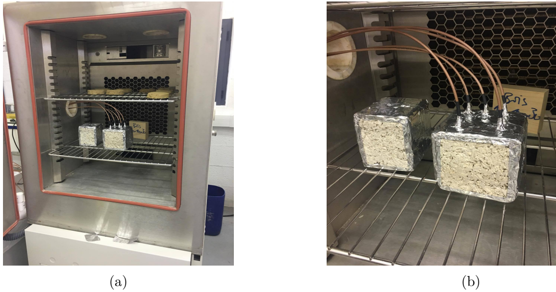
FIGURE 2.3 – The climatic chamber (a) and the tested sample (b)
