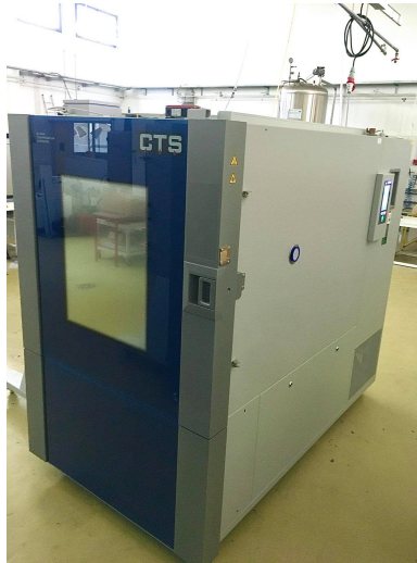
FIGURE 3.4 – The climatic chamber used in tests.
