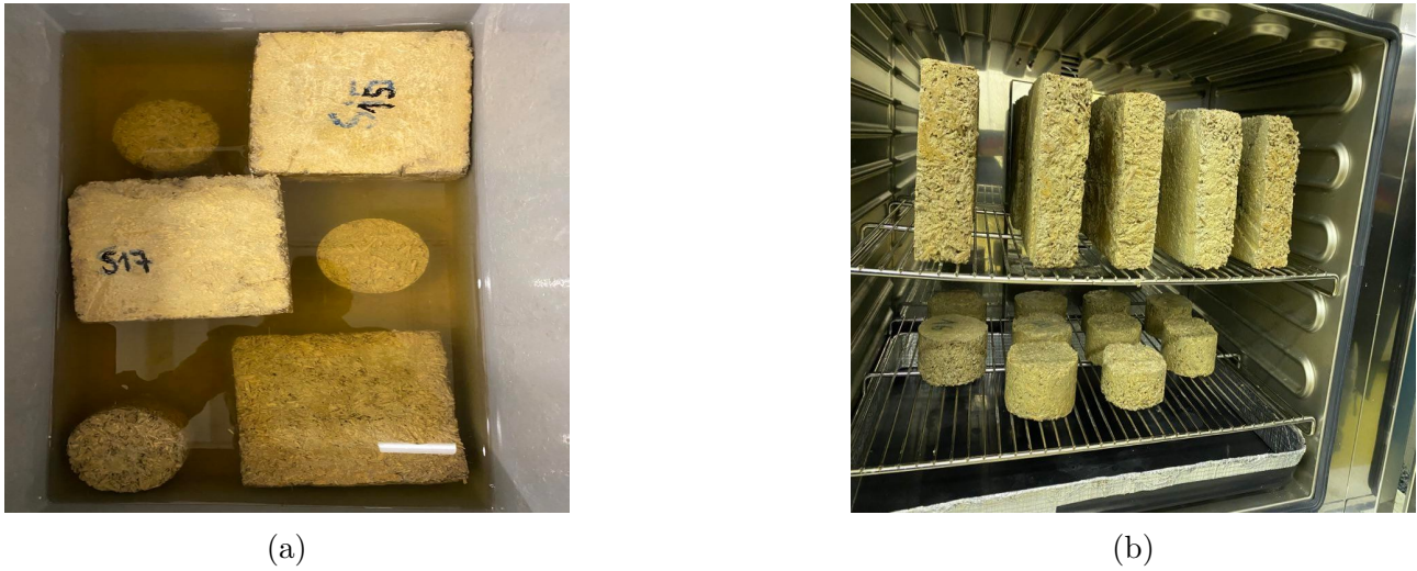
FIGURE 4.3 – Hemp concrete samples during immersions (a) and heat stress (b).
