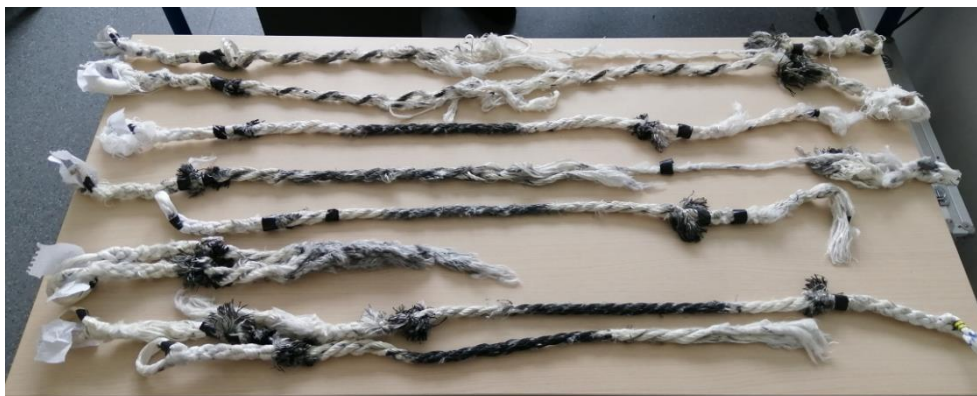
Figure 5.4 - 4T sub-rope samples after fatigue failure obtained during the MONAMOOR project
