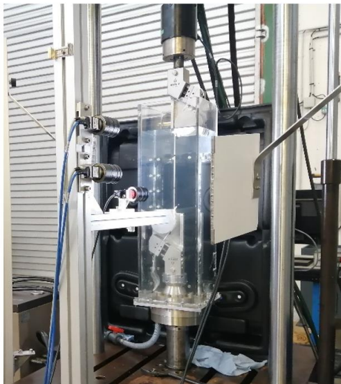
Figure 2.18 - Experimental set-up for cyclic tests in water with a plane-diopter tank and three cameras: two cameras for axial strain measurement; one camera for transversal strain measurement. Left: Test on rope-yarn scale. Right: Test on the strand scale (wood beams to block the actuator rotation).
