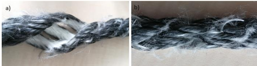
Figure 5.5 - Damaged 4T sub-rope after fatigue testing
