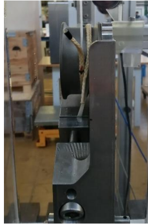
Figure 2.19 - Picture of the Vectran braided sheath (yellow) placed around the rope-yarns (white) for reducing the friction damage on contact with the capstan.
