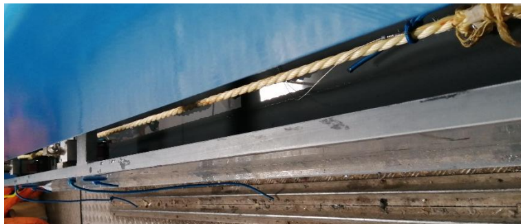
Figure 3.12 - 4T sub-rope sample after creep installed on IFREMER experimental set-up for the multi-relaxation test
