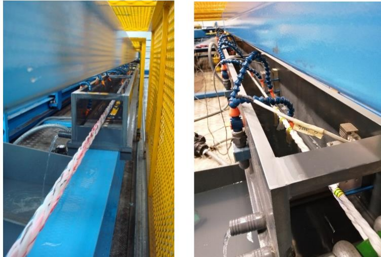
Figure 2.11 - Servo-hydraulic machine with 300 kN capacity: (left) 6-meter-long 7T sub-rope sample installed on the testing machine, (right) 4T sub-rope sample installed on the testing machine.
