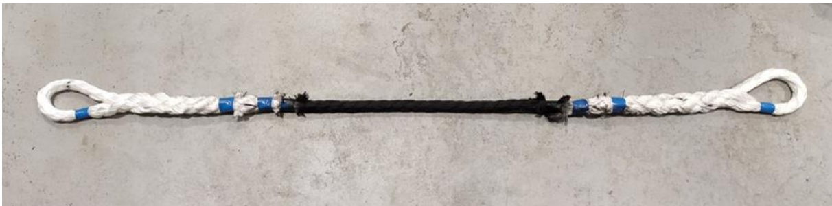
Figure 2.6 - 4T sub-rope sample with black paint on the gauge length to increase self-emissivity of the material
