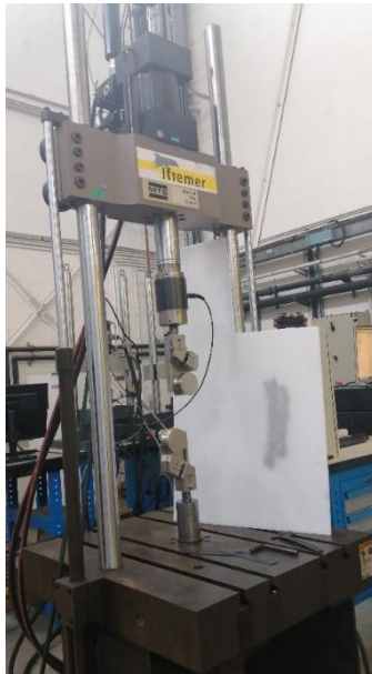
Figure 2.17 - Hydraulic testing machine used for the test on rope-yarns and strands in water: actuator of the machine is Figure 2.17above, hence, no risk of water damaging critical parts.
