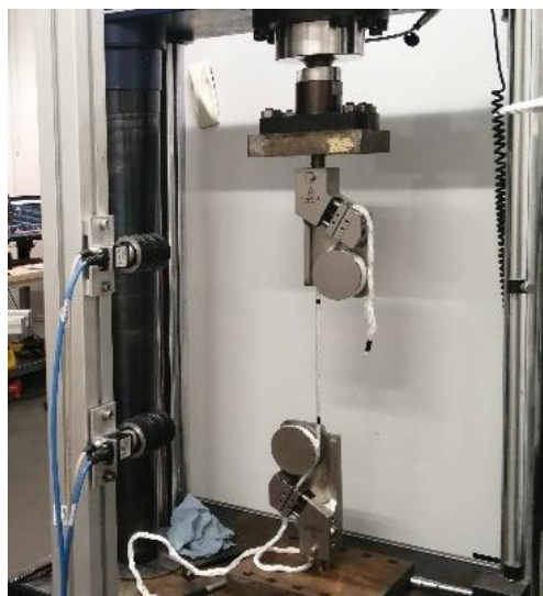
Figure 2.16 - Experimental set-up during a quasi-static tensile test on a strand with capstan grips. The same set-up is used for the rope-yarns.
