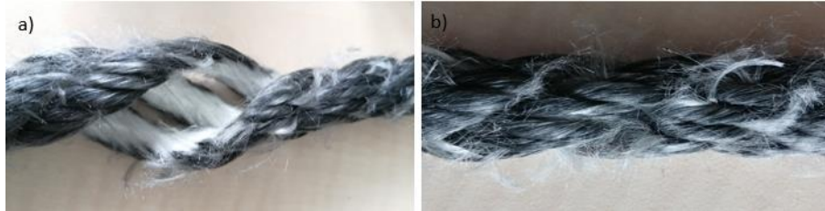
Figure 5.5 - Damaged 4T sub-rope after fatigue testing
