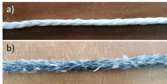
Figure 5.7 - Image of the samples analysed with X-ray tomography. a) Virgin sample. b) Sample after fatigue testing and failure in the eye-splice
