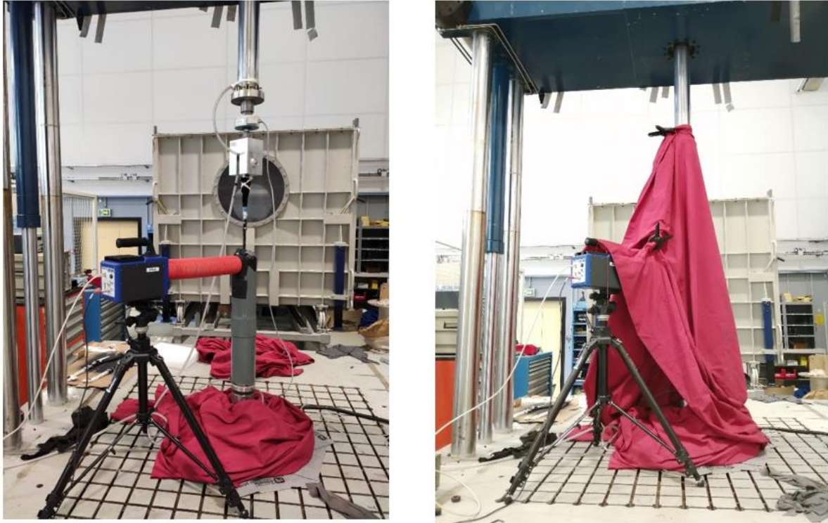
Figure 2.7 - Experimental set-up on the Servotest testing machine for fatigue test with self-heating measurement. a) plastic box and infrared camera installed. b) Sheet placed around the sample.
