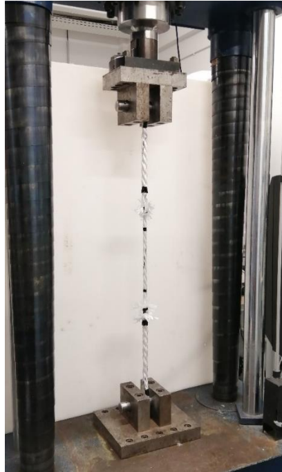
Figure 2.4 - Quasi-static test on 4T sub-rope samples: experimental set up using an electromechanical test machine
