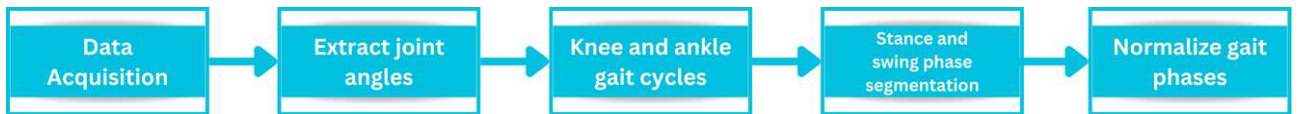
Figure 5.1: Flowchart of data pre-processing for experiment 2. We acquired trajectories of patient trials from the database and extracted all cycles from trials for knee and ankle joints. After that, we selected each cycle and segmented them into stance and swing phases. At last, we applied normalization to the phases.
