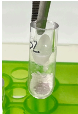
Figure S3-2. Intestinal sample prepared in 5-mL of 3% L-cysteine after the ultracentrifugation with 4 \times 10^5 G force for 2 hours. Thick mucus layer was observed on the top of the supernatant with a crystallized L-cysteine at the bottom and the wall of the tube, blocking the separation of LNC-50.
