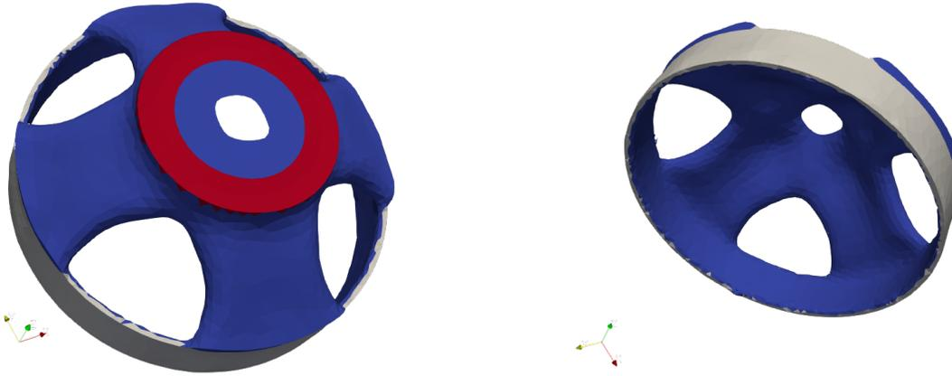
Figure 3.11: Optimal shape  $\Omega_4$  resulting from the polyhedron approach with  $N = 4$  vertices.
