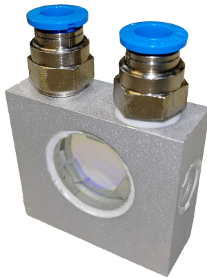
Figure 3.9: Picture of the ICAPS gas-cell used in this work, hosting the interferometer.
