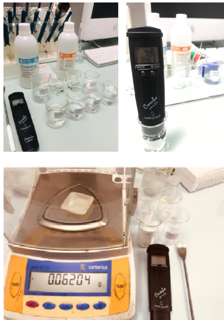
Figure 3.9: NaCl solutions preparation setup: precision balance, HI98129 conductivity meter and its cleaning and calibration solutions.
