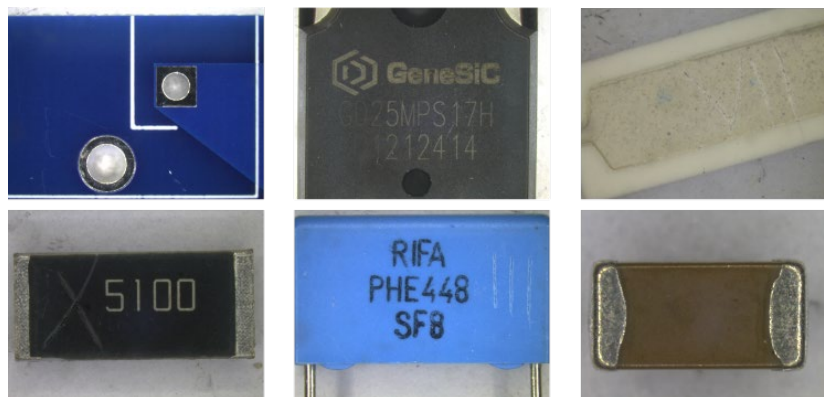
Fig. 6.20. Tested components before immersion, from top left to bottom right: PCB, diode, resistor 1, resistor 2, capacitor 1, capacitor 2.
