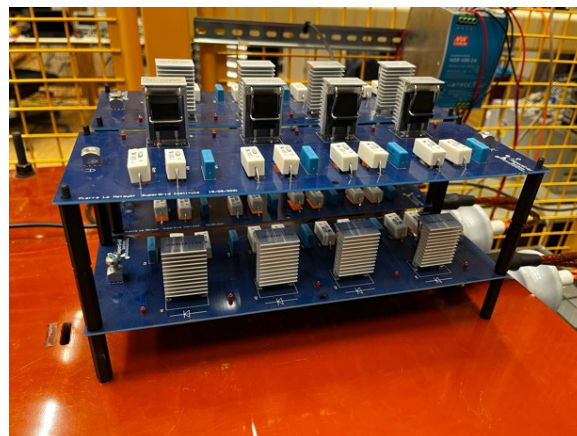
Fig. 6.4. Full-bridge rectifier composed of 4 diode assemblies (series connection of 4 diodes and individual RC snubbers).
