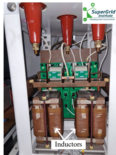
Fig. 7.6. Implementation of the DC-DC converter prototype, top) complete converter composed of inverter and oil tank, middle) oil tank, closed and open, bottom) elements inside of the tank
