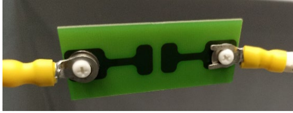
Fig. 6.14. Sample PCB with 3 mm gap and 70 \mu\text{m} thick traces
