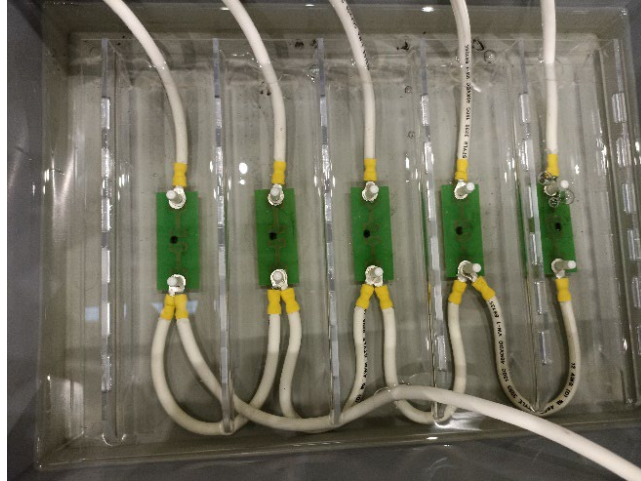
Fig. 6.15. Test set-up of the PCB samples, after a batch of tests (black spots where breakdown happened)
