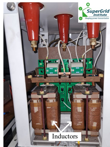
Fig. 7.6. Implementation of the DC-DC converter prototype, top) complete converter composed of the inverter and oil tank, middle) oil tank, closed and open, bottom) elements inside of the tank
