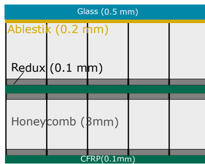
(a) Scheme of the full structure.
