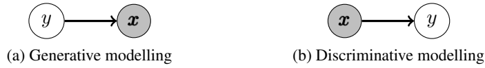
Figure 2.1 – The generative and discriminative modelling frameworks for clustering models. Observed variables are shaded.
