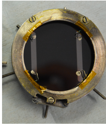
Figure 2.4 A photograph of the custom sample holder with Cu connection pins used for real-time resistance measurements with a Si wafer with the pre-deposited Ag electrodes. Two pins are connected to each electrode via 0.5 mm-thick cables, whose adhesion and connection to the electrodes is obtained using conductive silver ink.
