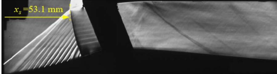
**Figure 2:** Schlieren photograph showing terminal shock controlled by bleed, from Chen et al. [20].
