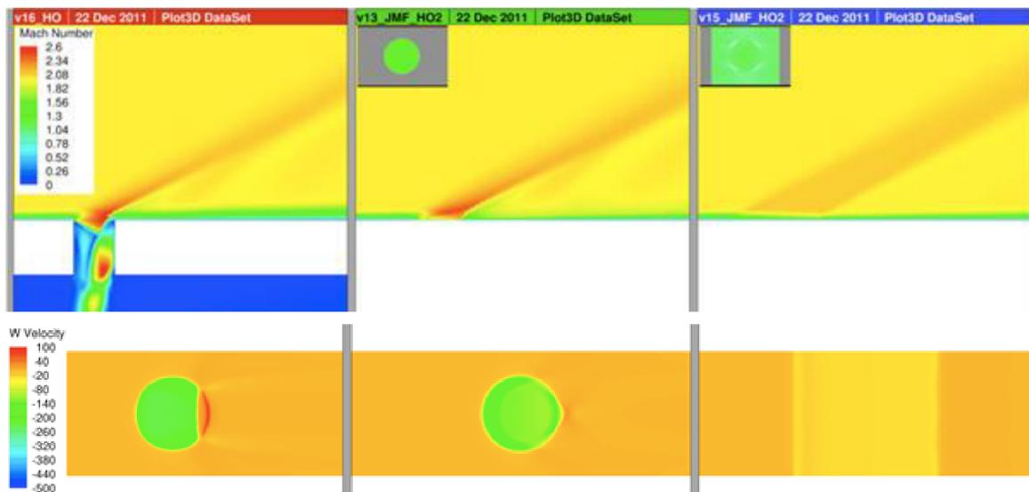
**Figure 1.46:** Mach contour field (top) and transpiration velocity (bottom) for reference simulation (left), pressure boundary condition (center), and model of Slater [98] (right), from Orkwis et al. [78].
