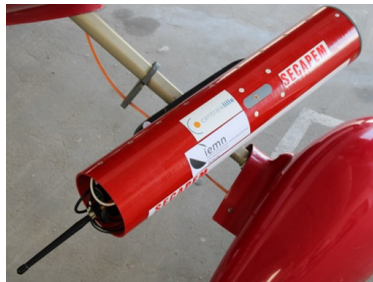
(b) POD installation on the microlight aircraft landing gear.
