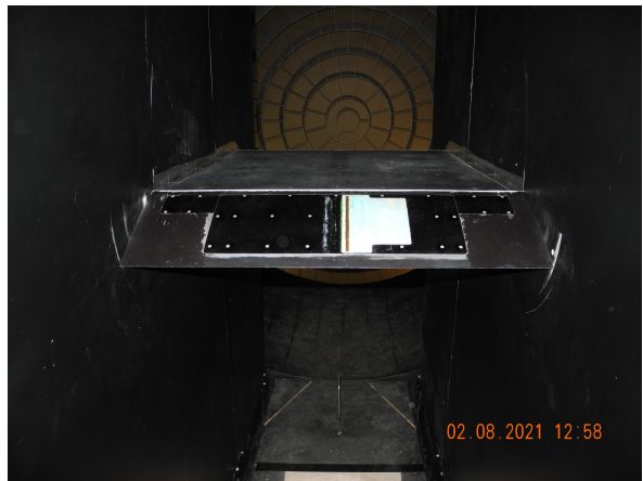
(b) Picture of the flap and hot films on its upper surface.
