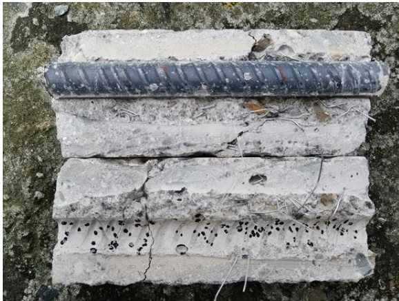
Figure 211 : bottom front bar of G3-07 sample after 30 cycles of wetting-drying cycles
