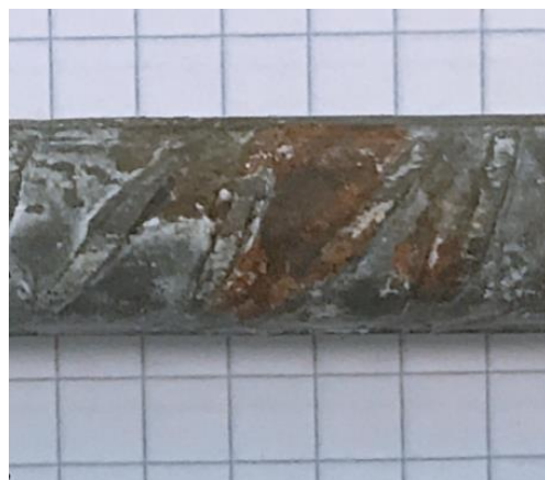
Figure 204 : Zoom of the corrosion at the location of the artificial crack after 4 cycles (top back bar of G3-10 specimen)
