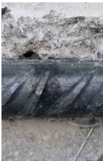
Figure 214 : corrosion stain visible between 2 ribs on top front bar G3-07 after 30 cycles
