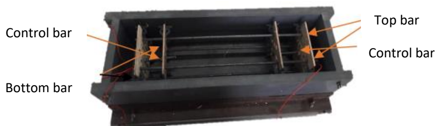
Figure 81. Photo of the special mold for casting concrete beam
