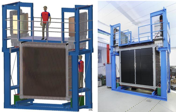
Figure 2.16: Left: Schematic layout of one NeuLAND frame supporting 15 double planes in total, here equipped with 13 double planes. A maintenance platform on top of the double planes allows for easy access to the readout electronics hosted in the boxes on both sides above the double plane, the high voltage supply boards are located in the lower left and right corners of each double-plane [93]. Right: Photo of the NeuLAND detector located in Cave C [94].
