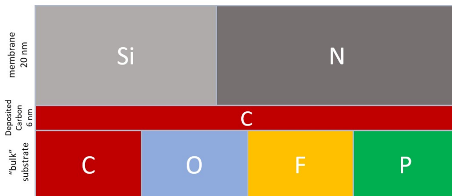
Figure 4.5: Model used for the SESSA simulations.
