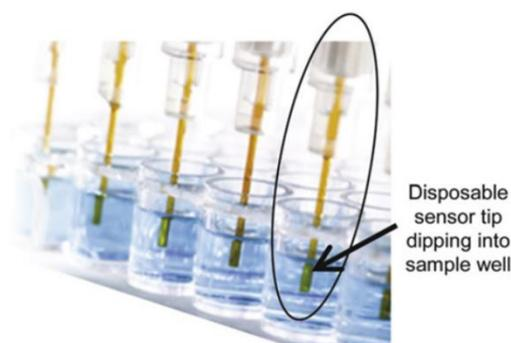
**Figure 36. Experimental setup of BLI technique**
