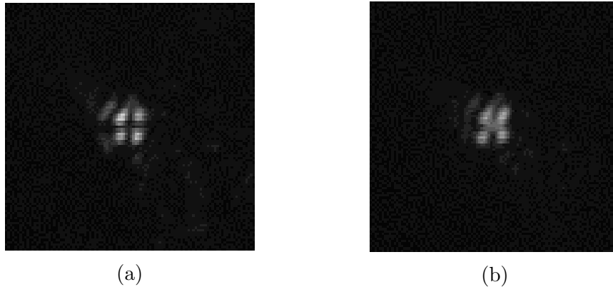
Figure 2.7: (a) Image of the beam partially reflected from the input surface of the fiber recorded by the camera after BS2. The characteristic clover-leaf pattern is observed. (b) In addition to this reflected beam, we see the white light that is coupled into the fiber when the LED is switched on. This allows for the easy alignment of the fiber core with respect to the center of the clover.
