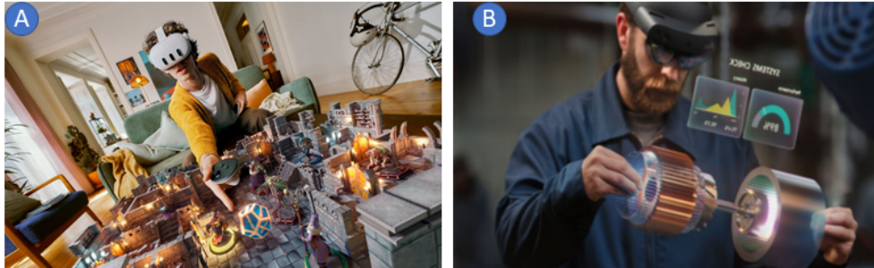
Figure 1.7 – Example of: A) Meta Quest 3 Video See-Through (VST) device [7], and B) Microsoft HoloLens 2 [8] Optical See-Through device (OST).
