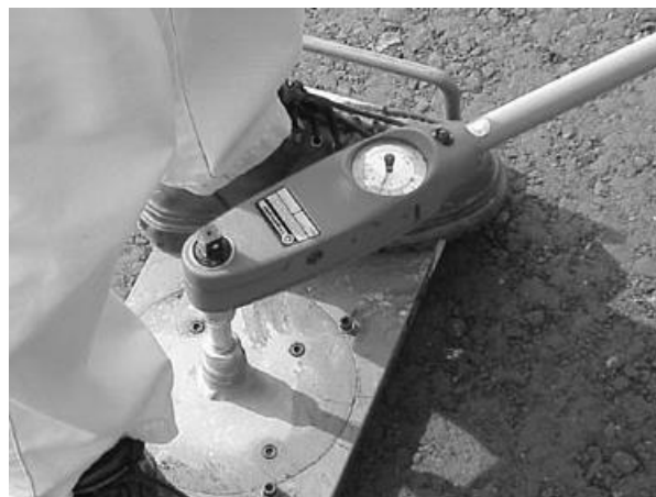
Figure 1.8: Torque bond test device in-situ (Attia, 2020)
