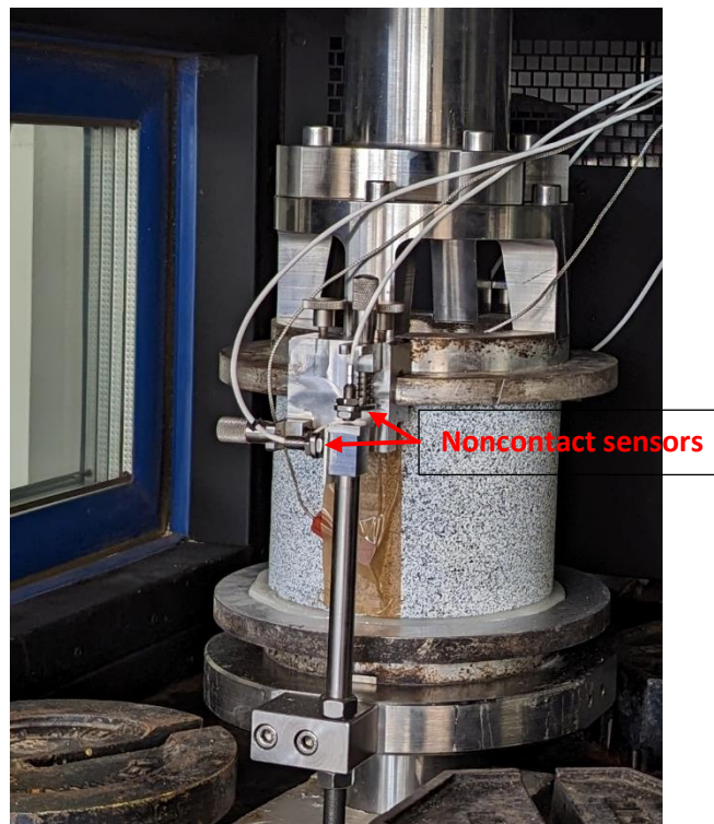
Figure 2.8: Two noncontact sensors placed in the front side used to measure axial displacement and rotation applied to the sample
