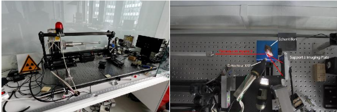
Figure 5.31 Left and right are the \mu -DRX and XRF portable laboratories of LAMS, credits: M. Bondetti, cf. LAPAUZE 2016:47-48)
