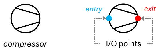
Figure 3-8. Graphic representation of a compressor with an entry point and an exit point.
