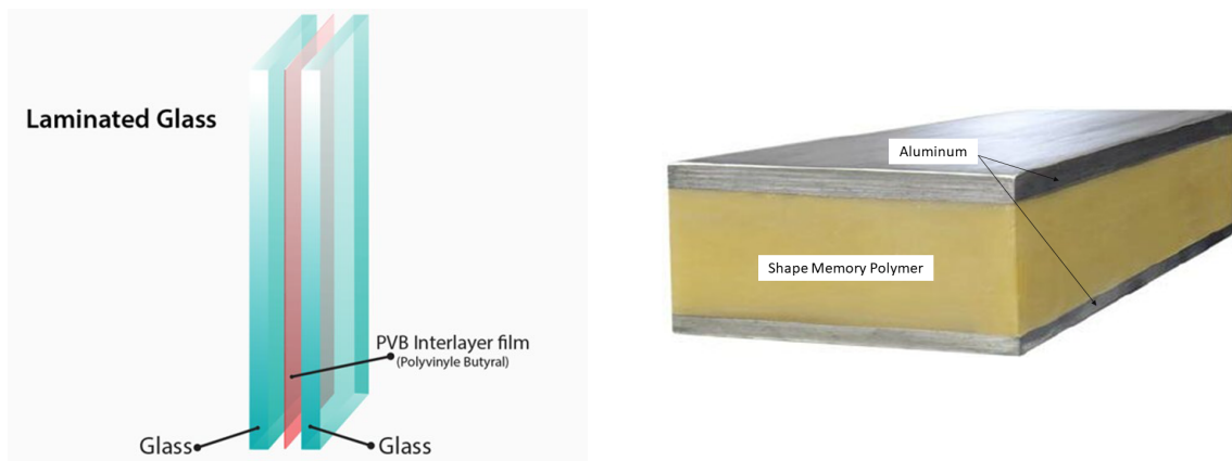
Fig. 1.3. Left: Laminated glass with PolyVinyl Butyral core [6]. Right: Sandwich plate with Shape Memory Polymer core [7].
