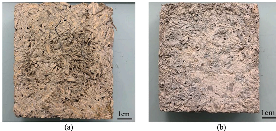
Fig. 4. (a) REF and (b) PCM hemp concrete samples for the thermal conductivity measurement.
