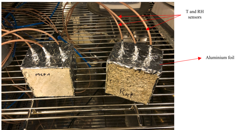
Fig. 7. REF and PCM hemp concrete samples for the thermal performances test and the position of the RH and T sensors.
