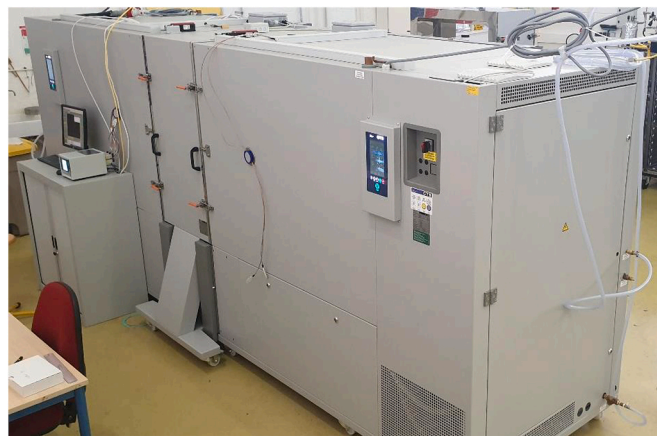
Figure A-3. C-40/1000/S – C-20/1000/S bi-climatic chamber from CTS GmbH for the hygrothermal test.
