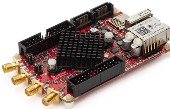
Figure 55 - The Red Pitaya STEMLab 125-14 SDR board.
