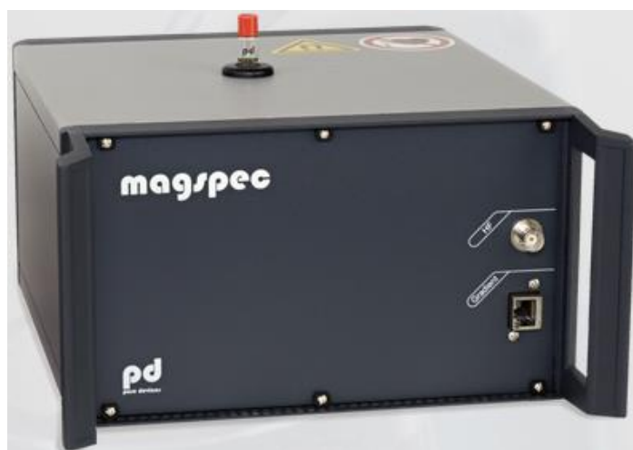
Figure 50 - Pure Devices magspec module consisting of a permanent magnet, a receiving coil, and shimming coils. Modified. [4]
