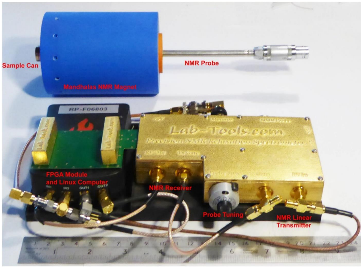
Figure 15 - Lab-Tools Mk3 NMR Relaxation Spectrometer with a Red Pitaya STEMLab 125-14. Modified. ([120], [121])
