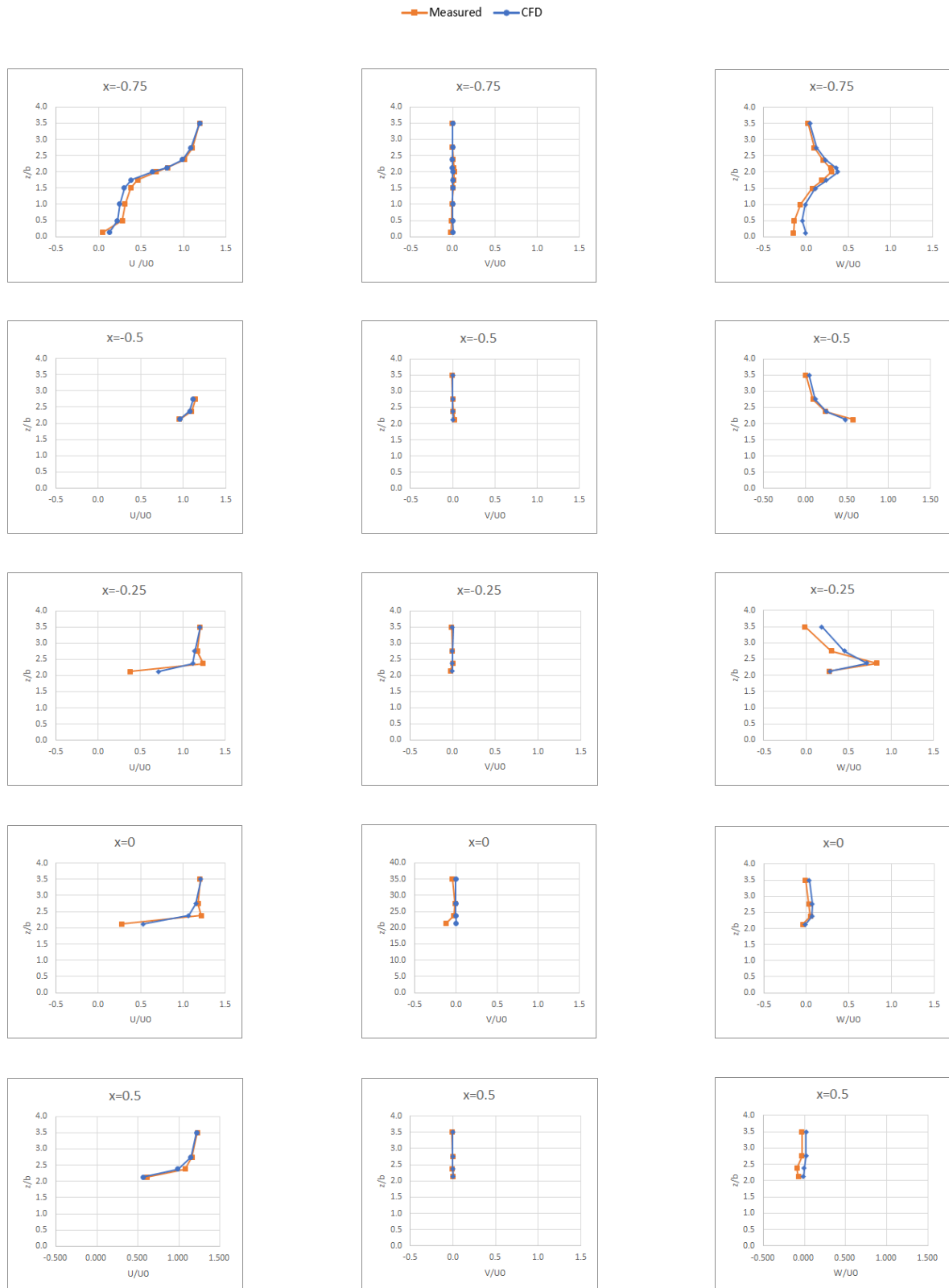
Figure 3.17: Wind profile for XZ vertical section (Part I : from x = -0.75b to 0.5b ). Average RNMSE on x = 0.89 , on y = 7.08 on z = 1.70 . Average error relative to U_0 on x = 9.6\% , on y = 0.9\% on z = 4.9\% .
