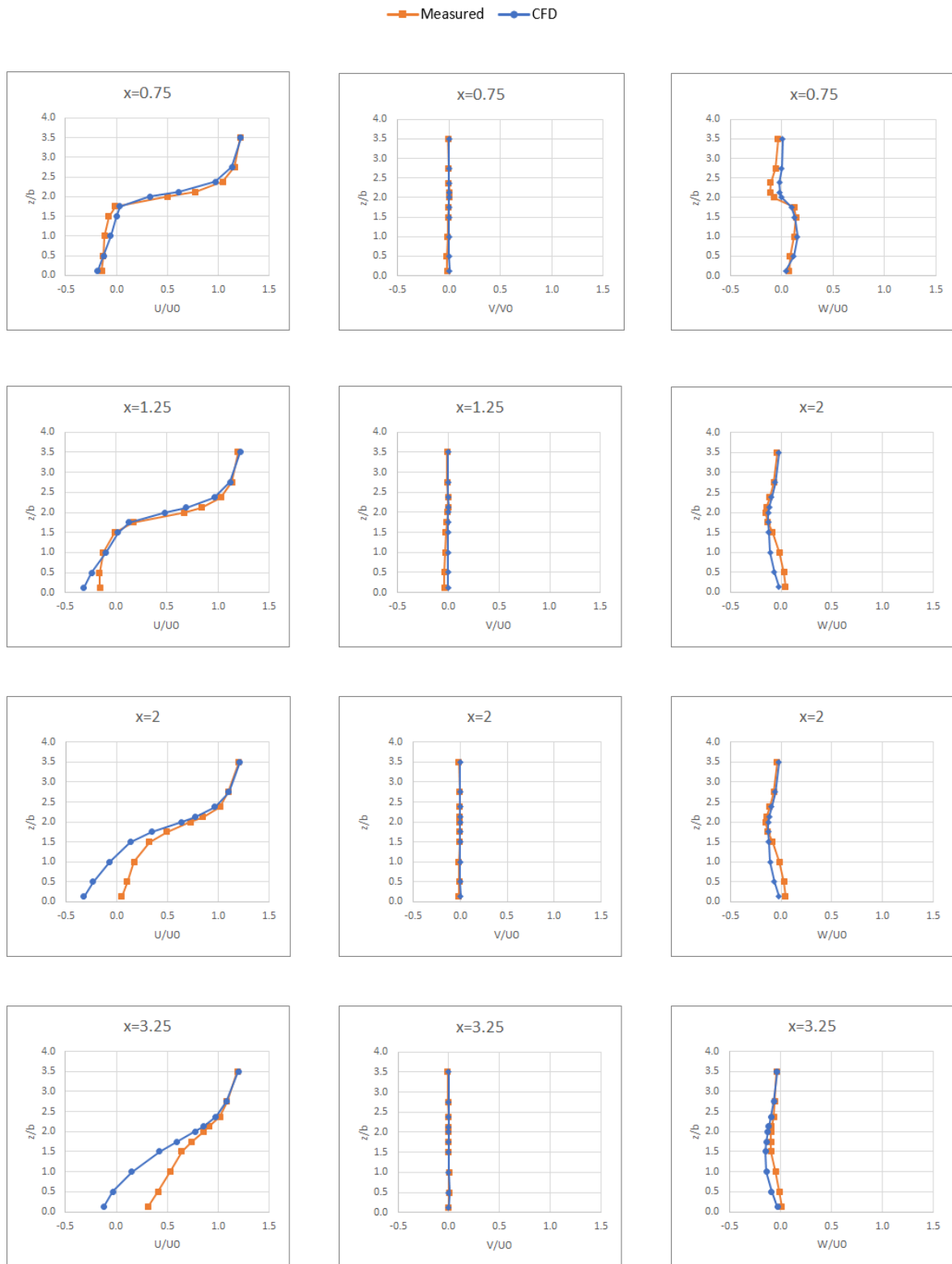
Figure 3.18: Wind profile for XZ vertical section (Part II : from x=0.75b to 3.25b ). Average RNMSE on x = 0.89 , on y = 7.08 on z = 1.70 . Average error relative to U_0 on x = 9.6\% , on y = 0.9\% on z = 4.9\% .
