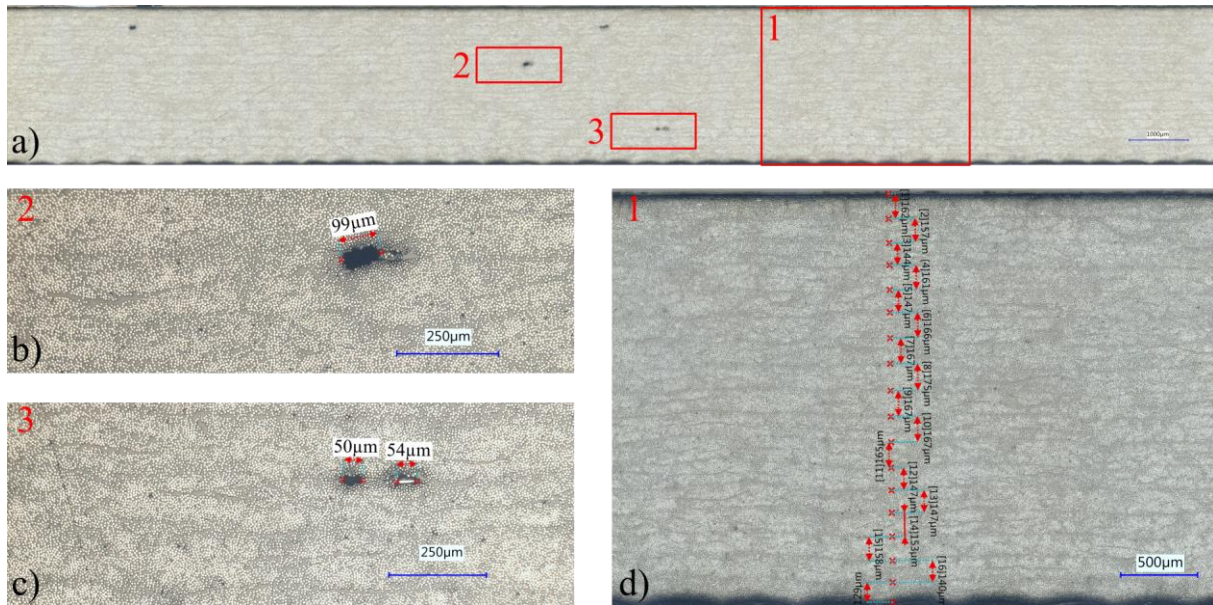
Fig. 2.12. Microscopic views of UTS17 samples under coaxial lighting; a) assembly for UTS17 sample; b) close-up view of region 2 with measurement of void; c) close-up view of region 3 with measurements of voids dimensions; d) close-up view of region 1 with ply thickness measurements
