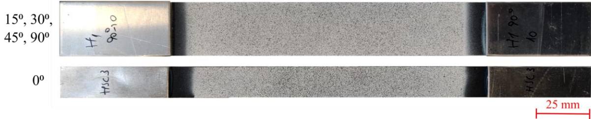
Fig. 3.4. Tensile test specimens with aluminum end tabs and speckle pattern
