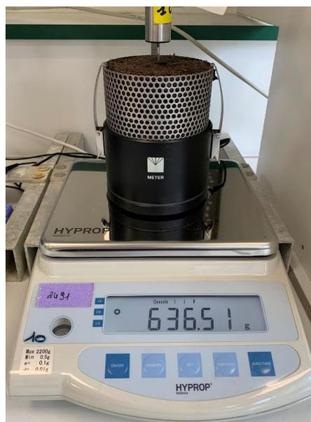
**Figure 11.** Shrinkage properties measurement with HyProp systems (Hyprop II, Meter Group Inc., USA) coupled with LVDT determining continuously water content, water potential and changes in total volume.
