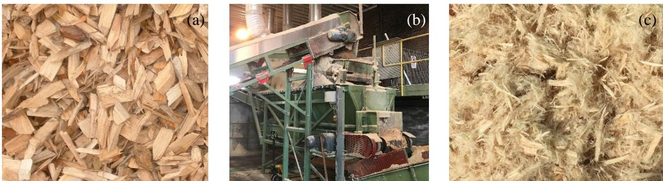
**Figure 7.** Defibration of wood pellets (a) into wood fiber (c) using a defibration tools (b).
