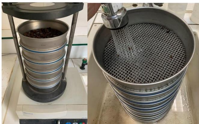
**Figure 13.** Wet sieving procedure for collecting derived particle size fractions from raw materials.
