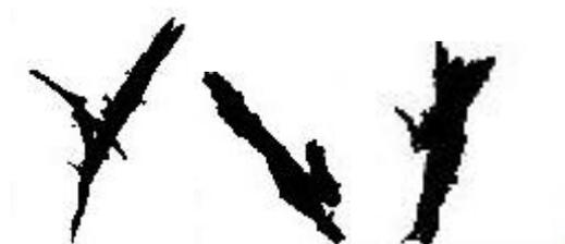
**Figure 3.** Wood fiber particles showing convex parts explaining discrepancy in various diameters assessing the width.
