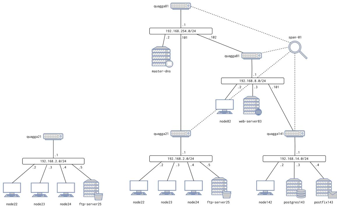
(a) Example of a sub-topology containing 3 Windows clients and 1 FTP server. (b) Example of a complete topology composed of 3 sub-topologies. The *span* captures the traffic of all gateways to simulate various probe positions afterward.
