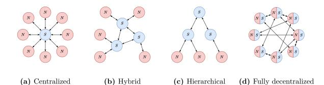
**Figure 2.4** – Different topologies for collaborative intrusion detection systems. Nodes are in red and marked as N, while servers are in blue and marked as S. Arrows represent connections between entities.
