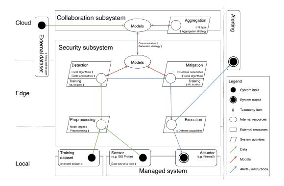
**Figure 3.9** – The proposed reference architecture for FIDSs. Figure from Lavaur, Pahl, *et al.*  $[Lav+22c] \odot IEEE 2022.$
