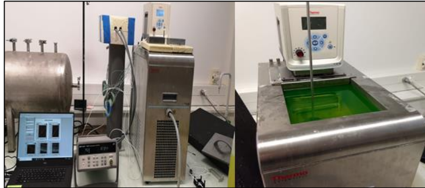
Figure 3.12: Hot bath technique for thermocouple calibration
