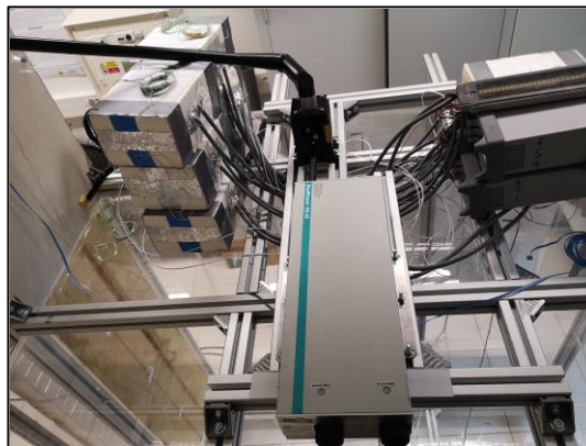
Figure 3.8: Aluminium framing for laser sheet system: (a) Scale model of laser sheet system (b) View of Laser sheet system installed on the ceiling of the room.
